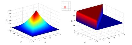
Fine scale Green's functions g' for linears in the diffusive  $(\alpha = 10^{-2}, \text{ left})$  and in the advective  $(\alpha = 10^2, \text{ right})$  regime;  $\alpha := \frac{\beta h}{2\kappa}$  is the mesh Peclét number.
