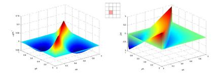
Fine scale Green's functions g' for quadratics in the diffusive  $(\alpha = 10^{-2}, \text{ left})$  and in the advective  $(\alpha = 10^2, \text{ right})$  regime;  $\alpha := \frac{\beta h}{2\kappa}$  is the mesh Peclét number.
