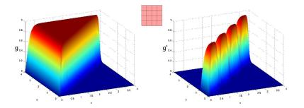
Comparison between the Green's function g (left) and the fine scale Green's function g' (right) for linear elements,  $\kappa = 10^{-1}$ ,  $\beta = 1$ , L = 4 and a grid of  $n_{el} = 4$  uniform elements.
