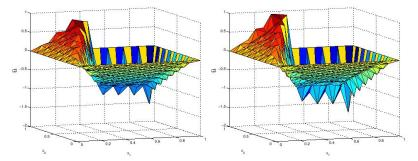
Coarse-scale component  $\bar{u}$  for the model problem (different mesh).  $\mathcal{P} = H_0^1$ -proj. (left) and  $\mathcal{P} = L^2$ -proj. (right).
