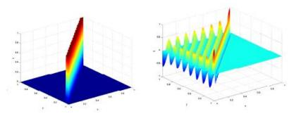
g' for the 1D problem and P1 coarse scales,  $\kappa = 10^{-3}$ ,  $\beta = 1$ , L = 1, 16 elem.;  $\mathcal{P} = H_0^1$ -proj. (left) and  $\mathcal{P} = L^2$ -proj. (right): in the latter case, g' is global and unattenuated.
