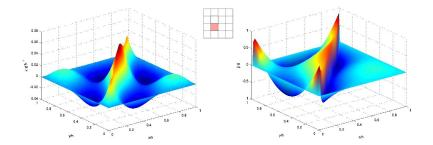
Fine scale Green's functions g' for cubics in the diffusive  $(\alpha = 10^{-2}, \text{ left})$  and in the advective  $(\alpha = 10^2, \text{ right})$  regime;  $\alpha := \frac{\beta h}{2\kappa}$  is the mesh Peclét number.
