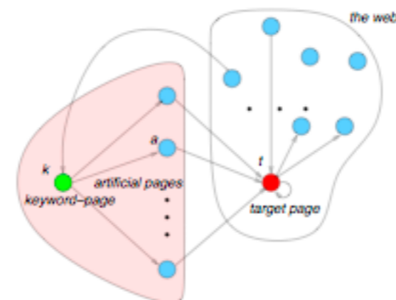
Figure 1: How to promote a web page by playing on the number of input links. A keyword-page is created which links to a set of artificial pages containing the selected keywords which, in turn, link to the target page.
