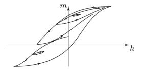
Tipical hysteresis diagram in ferromagnetism (h magnetic field, m magnetization).
