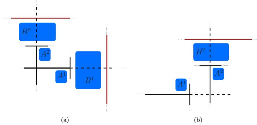
Fig. 10. T-junctions  $T^1$  and  $T^2$  for  $p$  and  $q$  even. (a)  $\text{ext}_{p,q}^e(T^1) \cap \text{ext}_{p,q}^e(T^2)$  is a vertex of the T-mesh. (b)  $\text{ext}_{p,q}^f(T^1) \cap \text{ext}_{p,q}^e(T^2)$  belongs to a vertical edge of the mesh.
