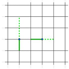
Fig. 3. Extensions for degree  $p = 2$  (horizontal) and  $q = 3$  (vertical). The dashed lines represent the face extensions.
